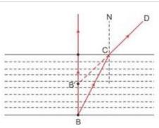
Let any object B is at the bottom of a pond. Consider a light ray BC from the object that moves from water to air. After refraction from the water surface, the ray moves away from the normal N along the path CD. The produce of CD appears from the point B' and a virtual image of the object at B appears at B'.
