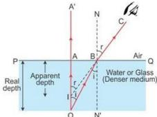
Consider a ray of light incident normally along OA. It passes straight along OAA'. Consider another ray from O (the object) incident at an angle i along OB. This ray gets refracted and passes along BC. On producing this ray BC backwards, it appears to come from the point I, and hence, AI represents the apparent depth, which is less than the real depth AO.
