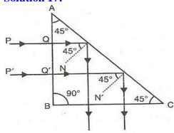
As shown in diagram, a beam of light is incident on face AB of the prism normally so it passes undeviated and strikes the face AC where it makes an angle of 45° with the normal to AC. Because here the incident angle is more than critical angle so rays suffer total internal reflection and reflect at angle of 45°. The beam then strikes face BC, where it is incident normally and so passes undeviated. As a result the incident beam gets deviated through 90°.
