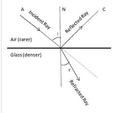
Diagram showing the refraction of light from Glass to Air
