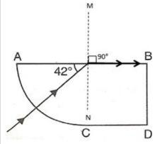
The angle of refraction will be 90° because the ray is incident on the glass at its critical angle.
