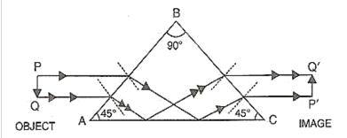
It is an erecting prism which is used to erect the inverted image without producing deviation in its path.
