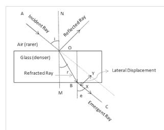
(b) Angle of incidence (i) and angle of refraction (r) are marked in part (a). Refractive index  $(\mu)$  of glass is related to the angles as
