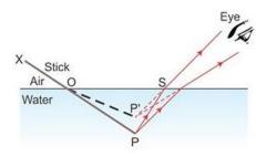
A stick partially immersed in water in a glass container appears bent or raised as shown in figure above. This happens because the rays appear to come from P' (which is the virtual image of the tip P of the stick) due to refraction from denser medium (water) to rarer medium (air) at the surface separating two media.
