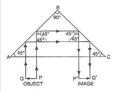
This action of prism is used in binocular.
